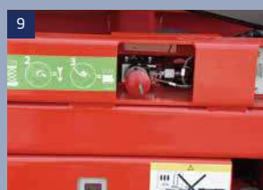
Manual lowering valve: When the operation system failed or the battery power is too low to let the platform decline, we can use this valve to lower the machine
