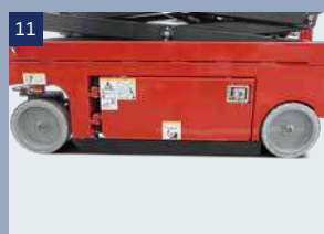
Manual lowering valve: When the operation system failed or the battery power is too low to let the platform decline, we can use this valve to lower the machine
